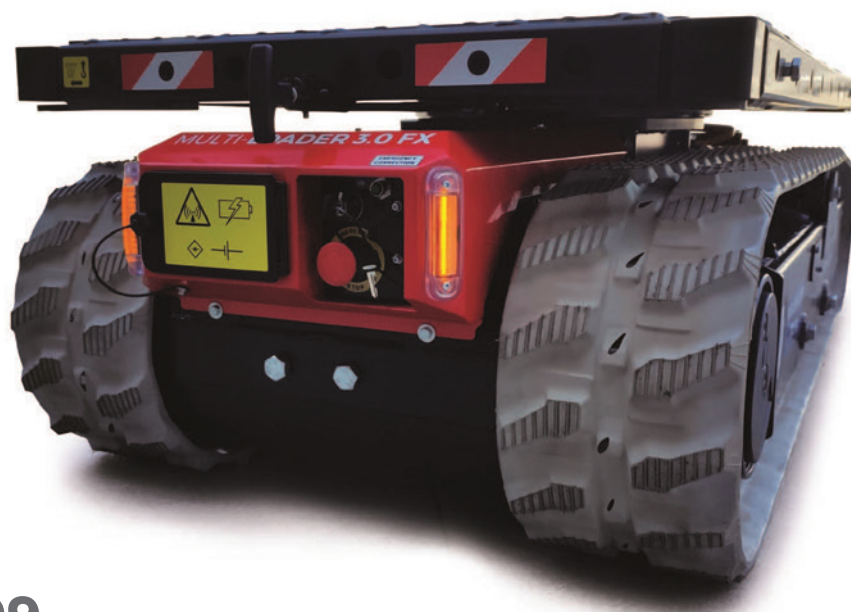
The ML 3.0 FX is a powerful and versatile flatbed truck carrier with a load capacity of 3,000kg.
