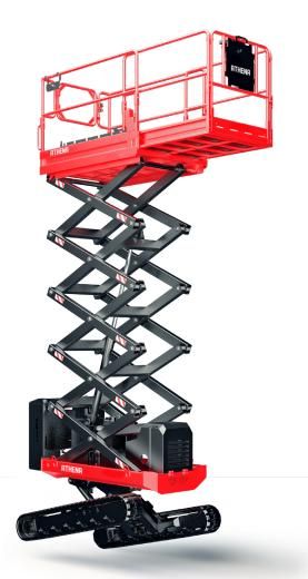
The ATHENA 1090 EVO bi-levelling scissor lift is able to operate on an incline of up to 20° and now can take you to a whopping 10 metre working height.
